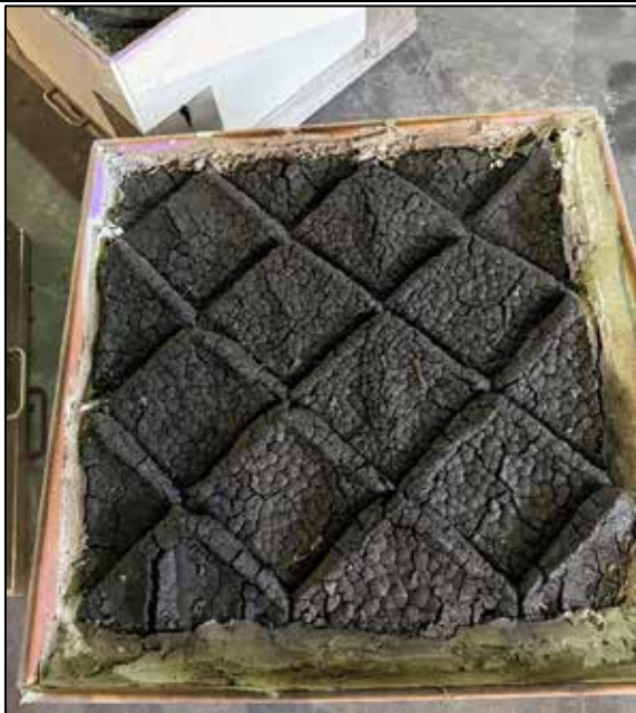
Figure 15: Damage investigation on the surface of the specimen
