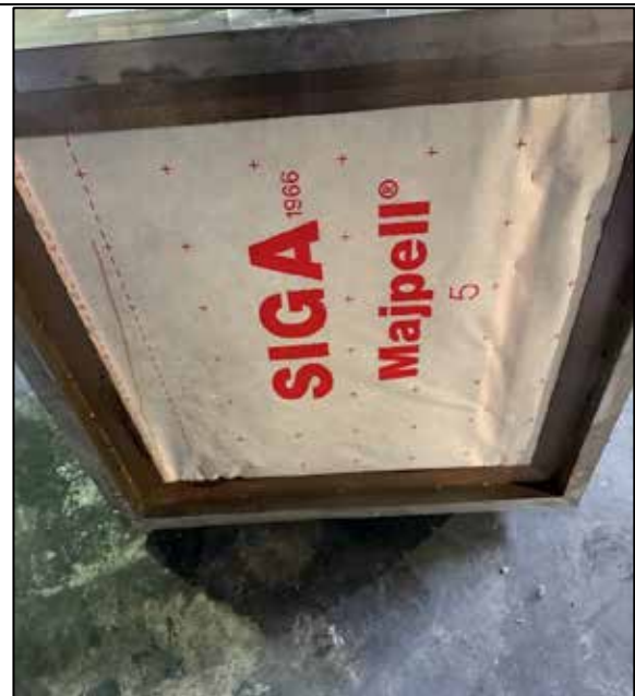
Figure 8: Damage investigation on the non-exposed side of the specimen
