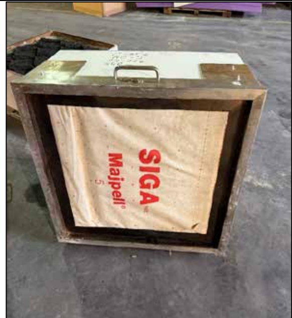
Figure 16: Damage investigation on the non-exposed side of the specimen
