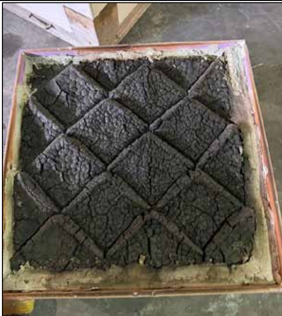
Figure 11: Damage investigation on the surface of the specimen
