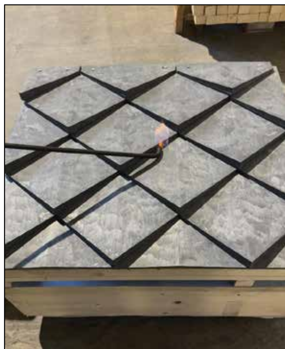
Figure 2: Sample during the application of the burning brand.
