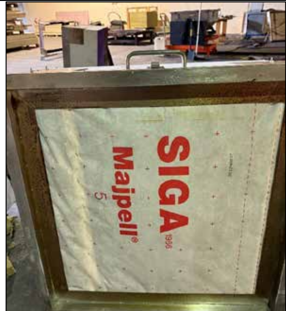
Figure 12: Damage investigation on the non-exposed side of the specimen
